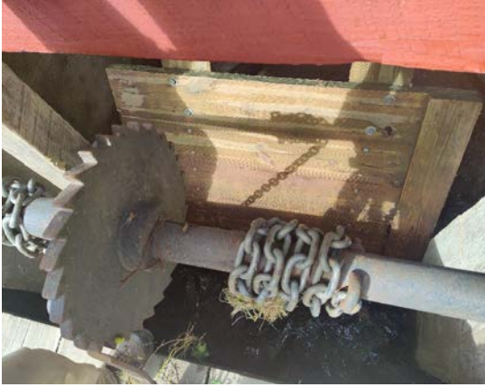
Inner workings of a waste gate
